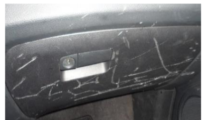
Diepe krassen dashboardklep
